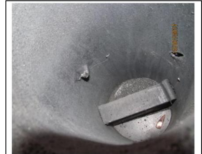
Figure 4: Shot 1 Stopped inside Gun mount.
